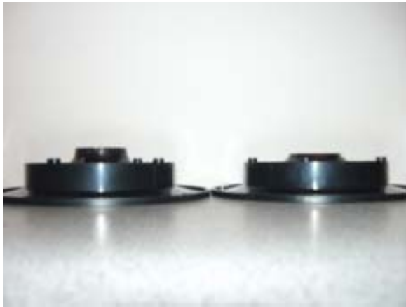
Pic 1.17 The Waveguide is shortened The picture shows the original and the 5mm shortened Waveguide. This can be done using file.
