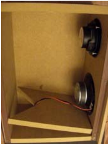
Pic. 2.13 chosen enclosure The triangle cut out in the board suppresses air motion noise.
