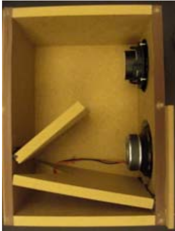
Pic. 2.15 Board To suppress standing waves in the enclosure a board is used.
