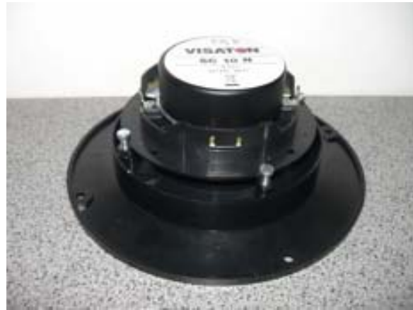
Pic 1.18 The Waveguide and tweeter The Waveguide is screwed to the tweeter. To do this you have to make notches in the mounting plate of the tweeter.
